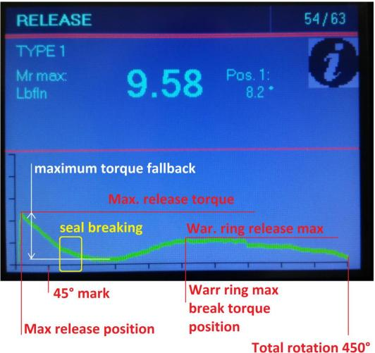
Figure 1 - Complete release process on a Torque-angle graph
