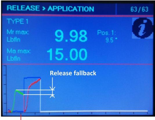
**15°mark** Figure 2 – Release>Application test with stop release on fallback
