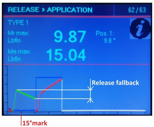
Figure 3 – Release>Application test with stop release on rotation
