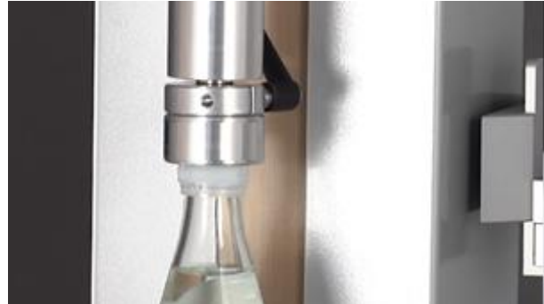
Ribbed chuck on competitor's tester – chuck and cap ribs must be synchronized
