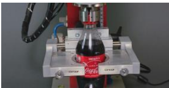
Pneumatic clamp on Sure Torque
