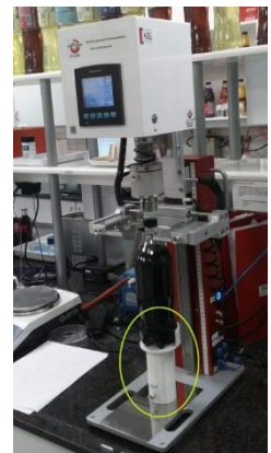
Ribbed chuck on competitor's tester – chuck and cap ribs must be synchronized
