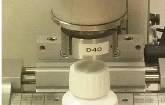
Pneumatic chuck on Sure Torque is capable for universal grab regardless rib position
