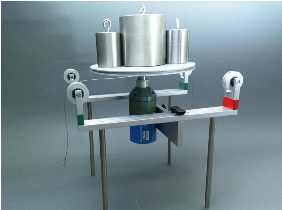
11. Remove the weight! Actual torque should be 0 Lbf and actual force should be 0 Lb
