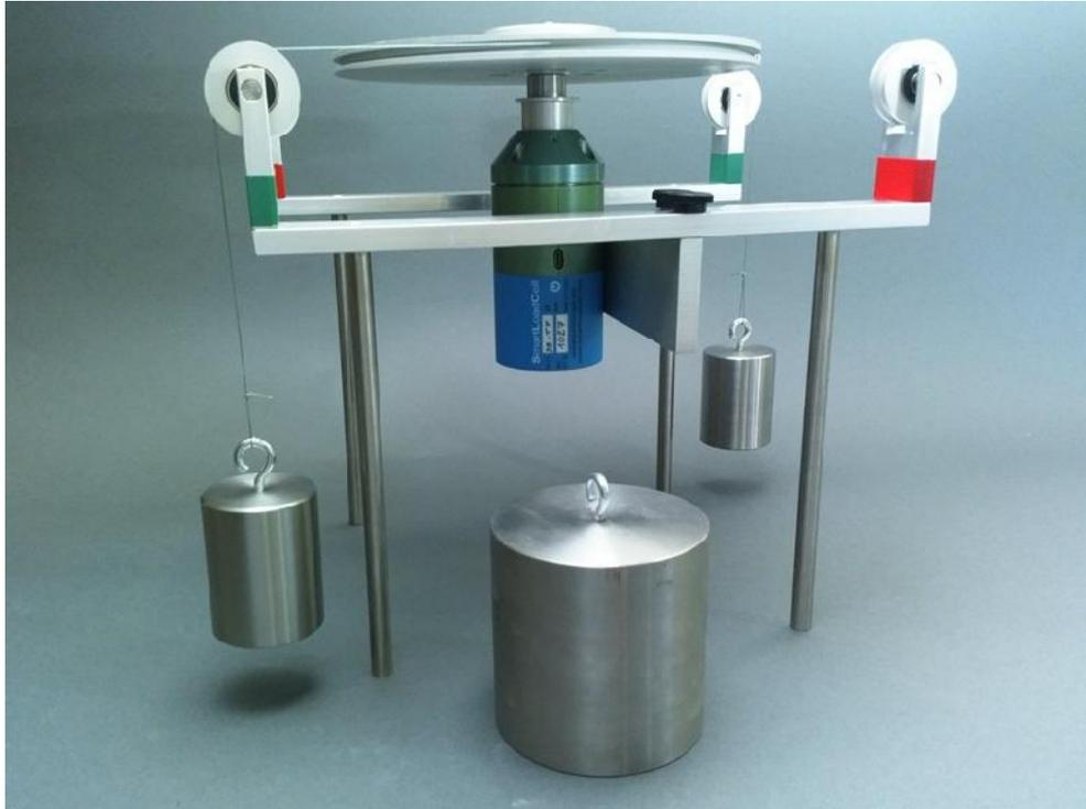
7. To check FORCE calibration place the big, 10 Lbf weight on the middle of the disk. You should read 16 Lbf/in actual torque and 10 Lbf actual force.
