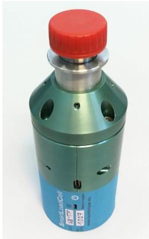
Smart Bottle is a Bluetooth wireless torque-force tester. SB-TF measures the dynamic chuck application torque and the top load on the capper machine even at normal production speed, during the production. Highest measuring speed is 200 Hz on each channel (torque, force).
