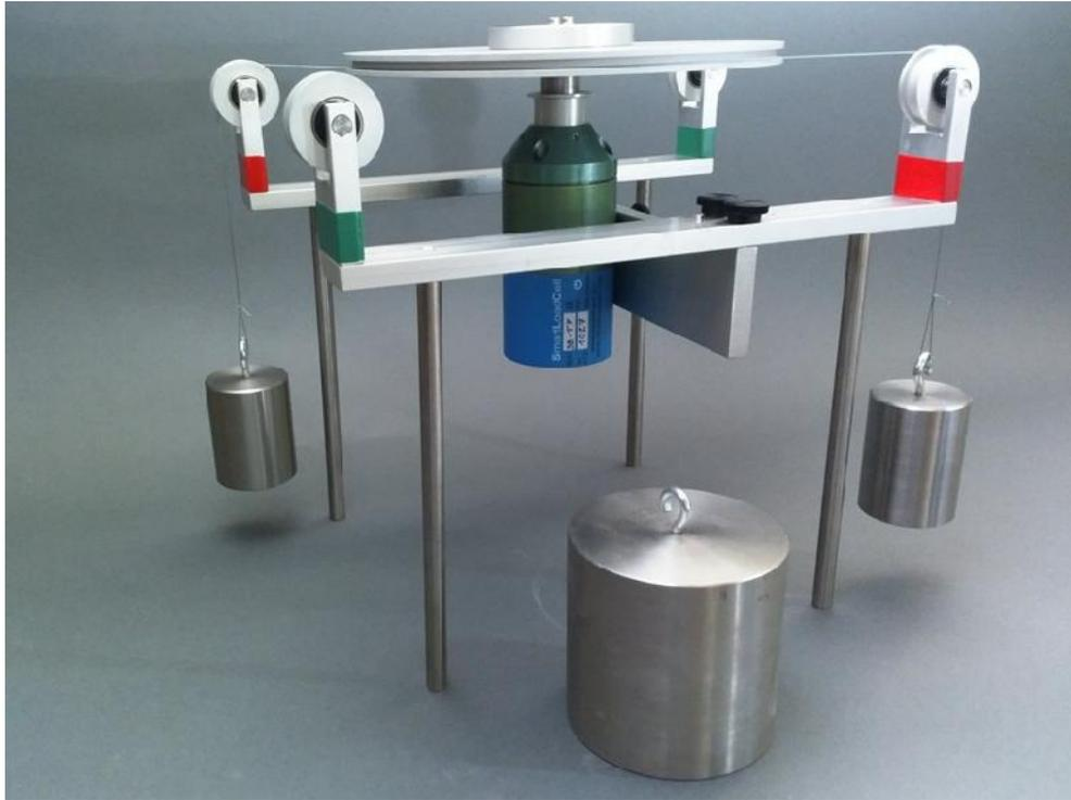
10. To check FORCE calibration place the big, 10 Lbf weight on the middle of the disk. You should read 10 Lbf actual force. You may add the 2 2Lb weights too, so you should read 14 Lb – **IMPORTANT: always put symmetric load on the Smart Bottle! Never use the 10 Lb weight for torque calibration!**
