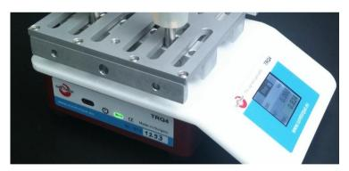
TRQ4 torque testers have built in LCD screens. They display the current and the peak values (Actual and Maximum). To change the setup of the screen, connect your device to an Android smartphone using the SmartLoadCell application.
