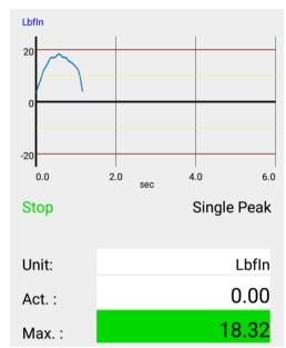
**Single peak** – Measurement stops automatic after the 1<sup>st</sup> peak.
