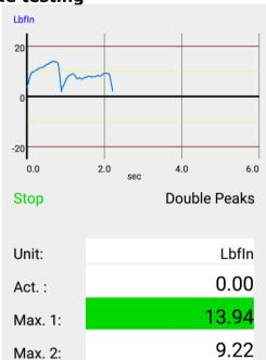
**Double peaks** – Measurement stops automatic after the 2<sup>nd</sup> peak.
